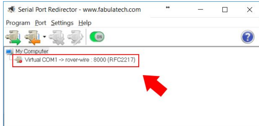
Figure 4: Virtual Serial Port present in Serial Port Redirector
